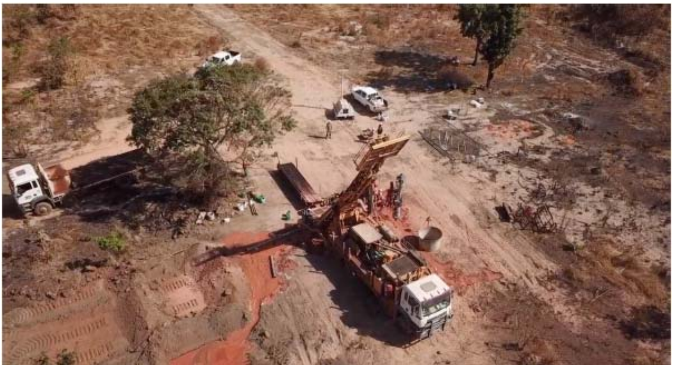
Figure 1: Photo of Diamond drilling Rig at Seko, Dandoko Project, West Mali
